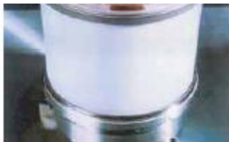
TH 2089B - Superklystron, extremely high output power (1.3 MW CW) and high efficiency.
